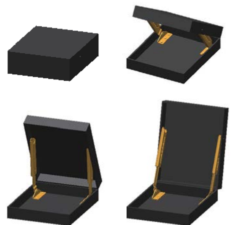
開啟時能五段定位或十段定位，關閉時需拉到底才可閉合 Pulls upwards to the end when the cover closes, then it closes downward.
